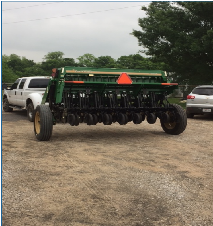
Figure 3 Ten foot No-till grain drill purchased with Section 319 funding
